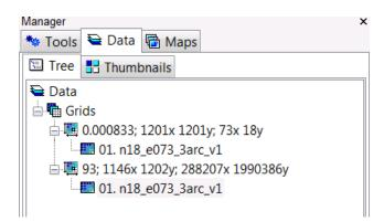
9. We are now ready to run a set of basic operations on the DEM via *Geoprocessing*  $\rightarrow$ *Terrain Analysis*  $\rightarrow$  *Morphometry*  $\rightarrow$  *Slope, Aspect, Curvature.* In this window, enter the current *'Grid sytem'* and *'Elevation'* as reprojected DEM and select the options as
