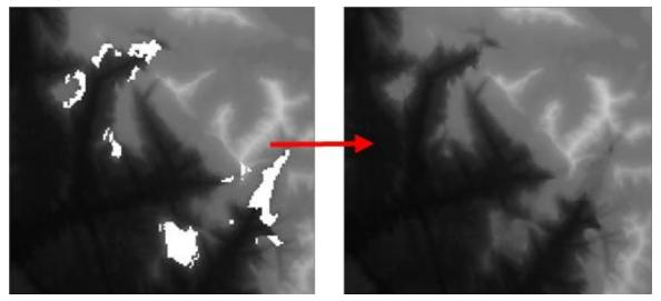
5. Now you can see that the gaps are filled by the estimated elevation values. Click the Description tab under Object Properties section. This will display the metadata of the DEM, some part of which is displayed below.
