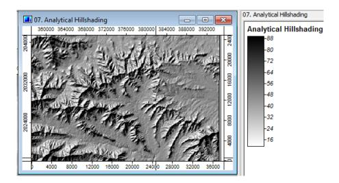
This simulates the shadow effect from a light source originating from the North West (315 degree) direction at an angle of 45 degrees from the horizontal plane.
